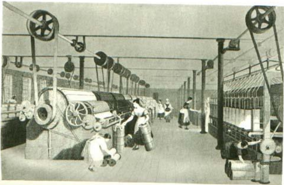
CARDING, DRAWING, AND ROVING AS IT WAS IN SAMUEL SLATER'S EARLY MILLS (From an old engraving)
